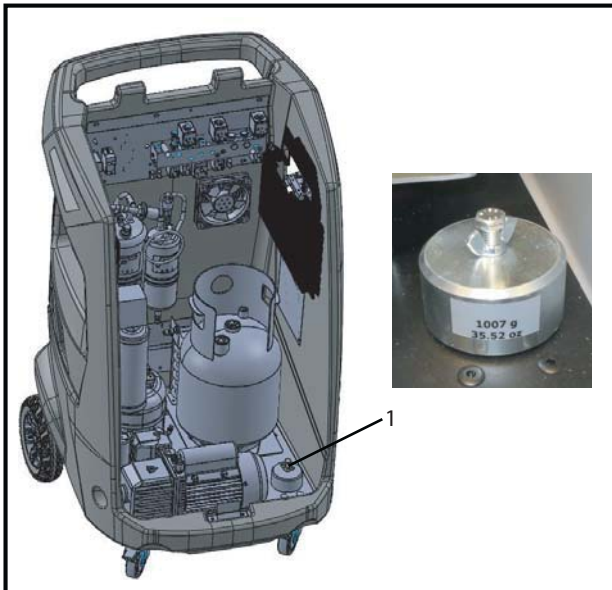
Fig. 33: Reference weight location
