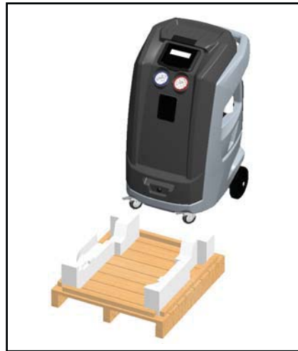
Fig. 11: Lowering unit from the pallet
