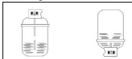
Fig. 13: Virgin refrigerant cylinder tank types
