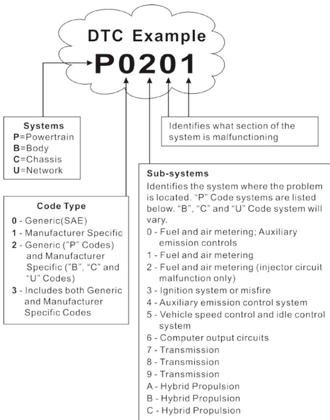
Figure 2-1 (P0201 - Injector circuit malfunction, Cylinder 1)
