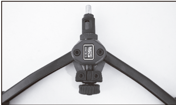
Riveter properly prepared for setting rivet nuts
