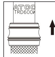
4. To lock wrench, release the LOCK RING.
