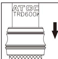
1. To unlock, pull the LOCK RING down and hold the handle GRIP.
