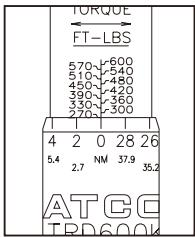
2. Rotate GRIP or SHAFT until "0" on the THIMBLE SCALE reaches the primary number of the desired torque value on the MAIN SCALE.
