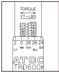
3. Continue rotating the GRIP if the desired torque value is between the primary numbers on the MAIN SCALE. Add the secondary number on the THIMBLE SCALE to the primary number on the MAIN SCALE to achieve the desired torque value.
