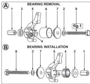
**BEARING INSTALLATION:** Identify the correct sleeve cap (7) to sit on the outside of the bearing housing and the correct diameter drift (3) to drive the new bearing into the housing. Assemble as shown in fig.1B. Keep the hub screw and nut well lubricated whilst driving the new bearing into the housing.
